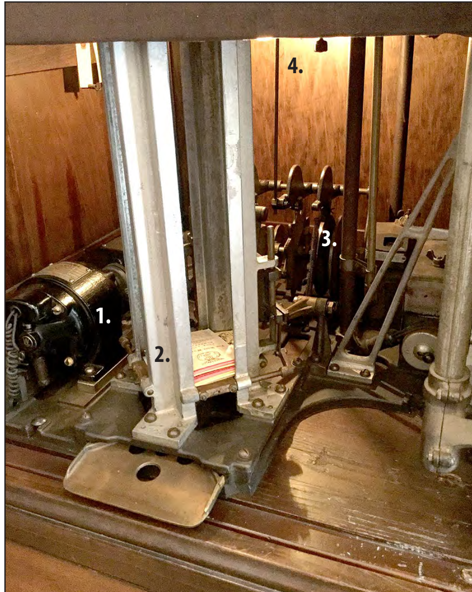
Interior of the Gent Grandmother Fortune Teller. Every machine is mechanically identical, with a strong, well-built mechanism made of cast-iron and bronze parts. 1. Westinghouse motor. 2. The card-vending mechanism, with bronze tray. The fortune card is delivered through an opening in the front door. 3. Bronze cams, which control all the movements. 4. Switchable interior work light for servicing the mechanism.
