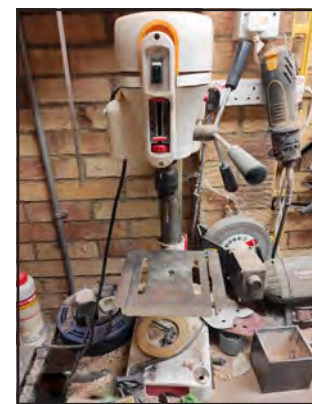
15. Drill press with depth gauge.
