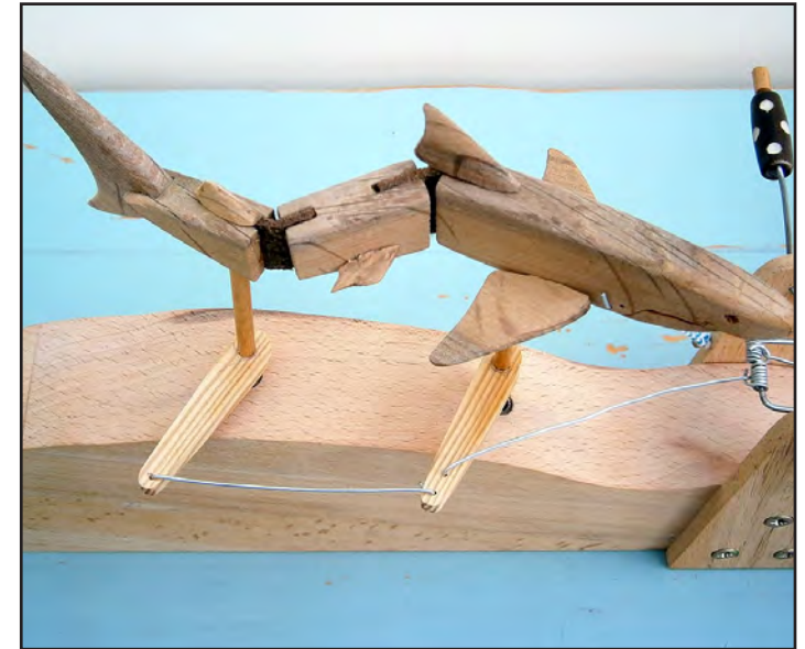
The flexibility and motion of the shark can be seen here, as well as the detail of the links to the crankshaft.
