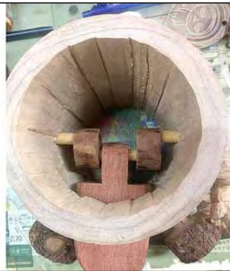
2. Looking down into the body of the automaton you can see how the crankshaft operates the tongue. The rotary motion is transformed to linear in-and-out motion.
