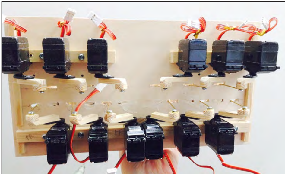
Twelve servo motors with wooden arms to push brass rods up and bring the birds to life.
