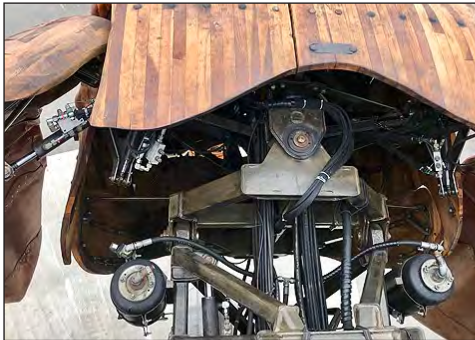
View of the head from the back, showing the mechanism operating the ears.
