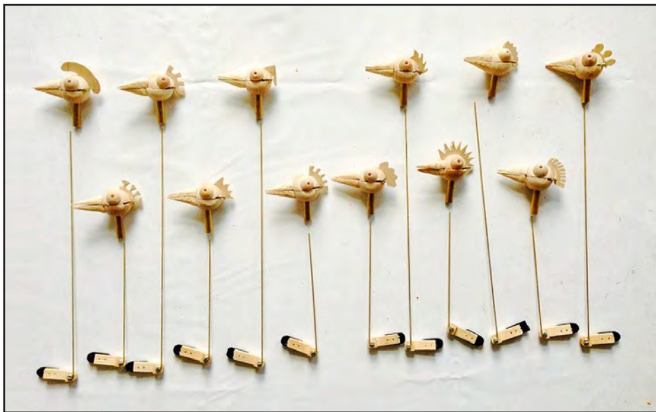
The birds' heads with their respective animating brass rods. The wooden arms mounted to the servo motors are seen below.
