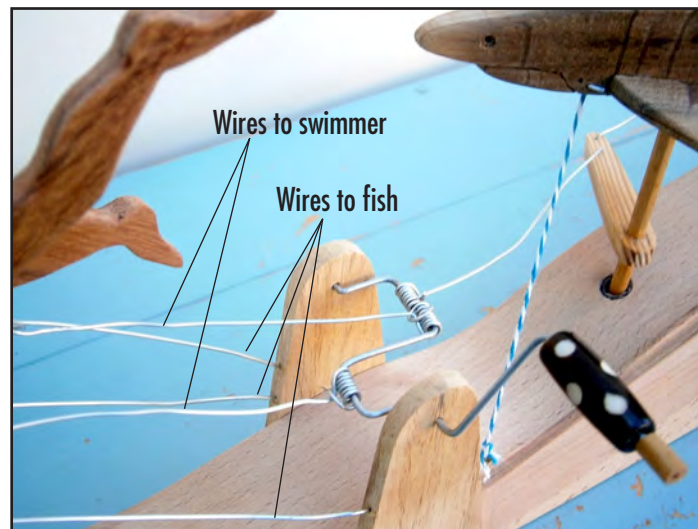
The extremities of the crankshaft movement are shown in these two photos. Two wire connections go forward to the swimmer (left), while the single connection goes back to the shark. The wire attachment to the fish is at the bottom left of the crankshaft supports. Note that, in the left photo, the swimmer's left leg is up and the shark's mouth is closed. The opposite is true in the right photo.
