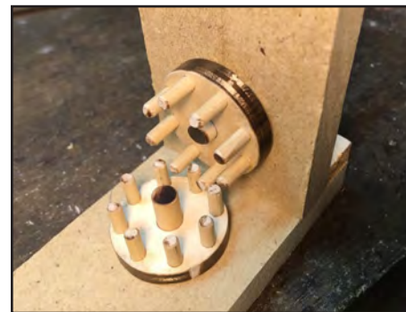
18. Gears being test fitted to determine their optimum positions on their shafts .
