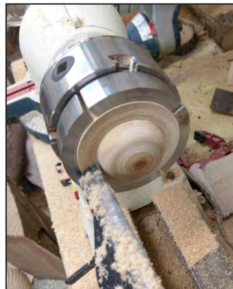
4. The eye being turned on the lathe. All of the automaton's parts were left in a natural wood finish.
