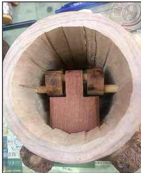
2. Looking down into the body of the automaton you can see how the crankshaft operates the tongue. The rotary motion is transformed to linear in-and-out motion.
