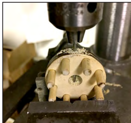
19. Gear being drilled for the retaining pin.
