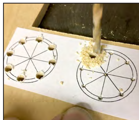
4. Holes must be drilled parallel to one another, preferably with a drill press.
