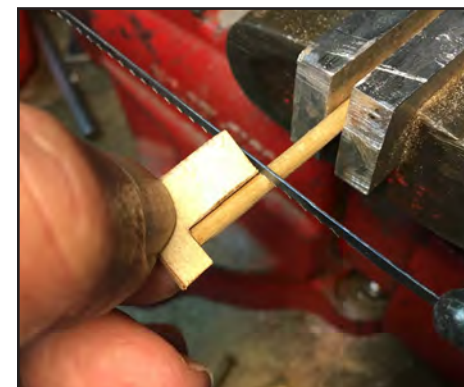
12. The gauge is used to position the saw.
