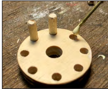
16. Glue is applied to the inside of the holes.
