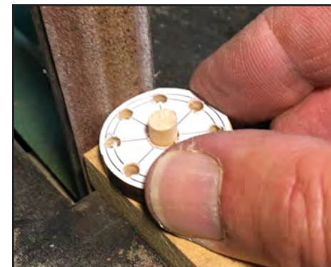
9. A wheel, mounted on the fixture, is sanded round on the belt sander.
