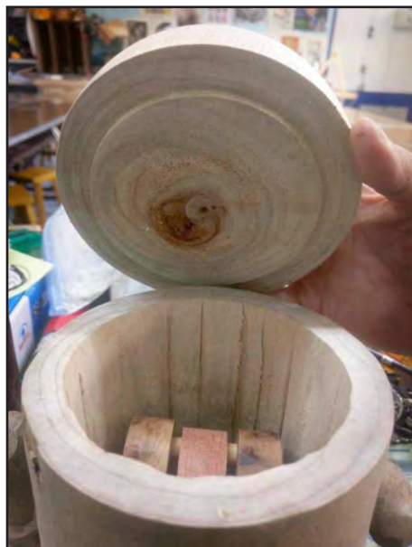
3. The Minion's top was also turned on the lathe. His headband disguises the joint.
