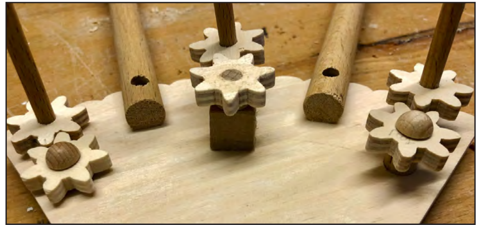
6, 7. Six small gears to drive the large gears are mounted to the rear part of the body. Note the different spacing of each pair of gears from the rear wall.
