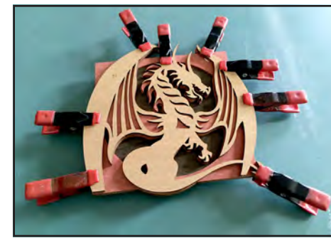
Parts clamped while gluing.
