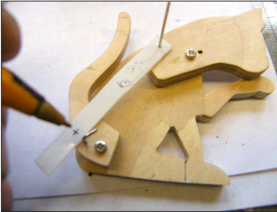
Head and tail are linked. The links pivot on short lengths of brass rod.
