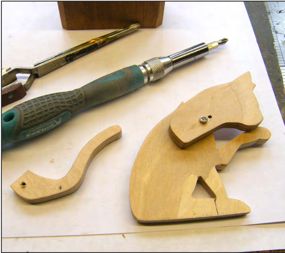
3. Head and tail are screwed to the body.
