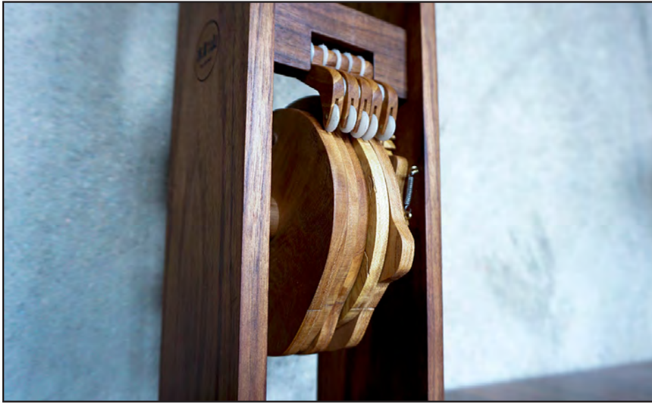
5. The automaton is controlled by five closely spaced cams.
