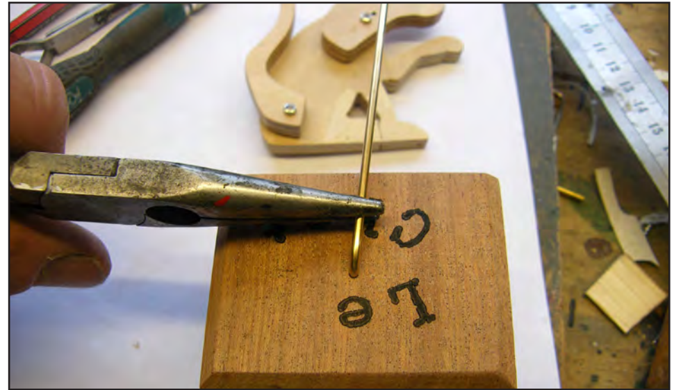
5. Once the rod has been inserted into the block, the crank handle is bent to shape on the front side of the block.
