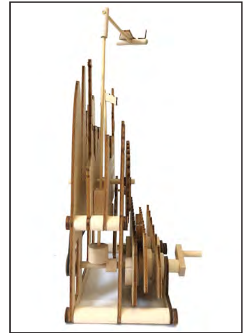
6. The London Cityscape sideways on, showing how the wave sections at the front ride on a series of cams. Ideally these need to be good and parallel. Otherwise they bind.
