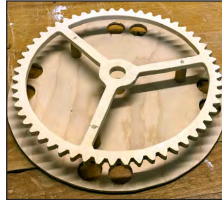
2. The "eyes" disc connected to its large gear with spacers.
