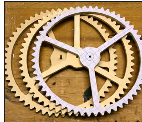
3. The three large gears were stacked and cut simultaneously on the scrollsaw.
