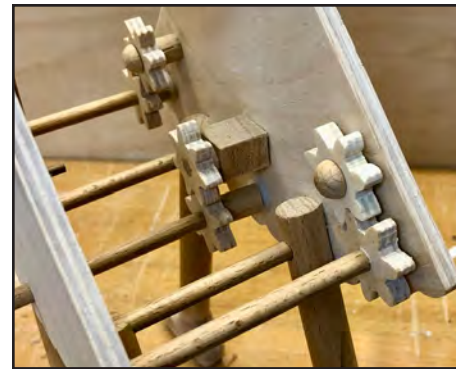
6, 7. Six small gears to drive the large gears are mounted to the rear part of the body. Note the different spacing of each pair of gears from the rear wall.
