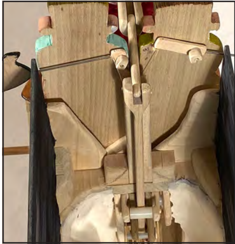
6. The mechanism that activates the speech bubbles as the virus's arm swings up.
