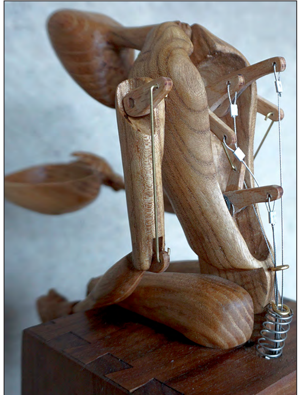
6. Wires from the struts, or cam followers, are connected to the figure's various body parts. The weight of each part returns it to its resting position.
