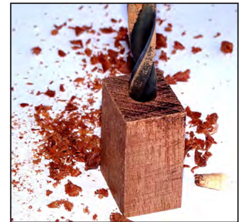
1. A hole is drilled through a block of wood that is to become the handle.
