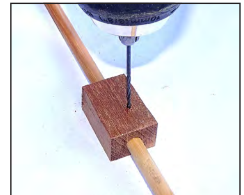
2. A smaller hole is drilled through the side of the block, just at the edge of the inserted dowel.
