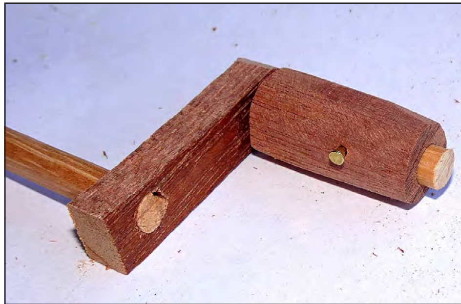
Handles that rotate on their shafts are more comfortable to use and add a bit of sparkle to the finished piece. The author tells how he makes his.
