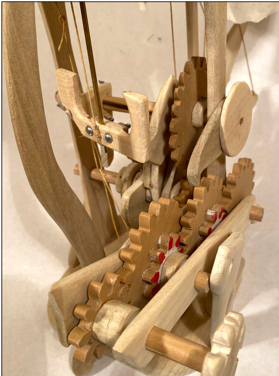
4. Closeup shot of the hand-cranked mechanism. Most parts are made of wood but the gears are 3D printed.
