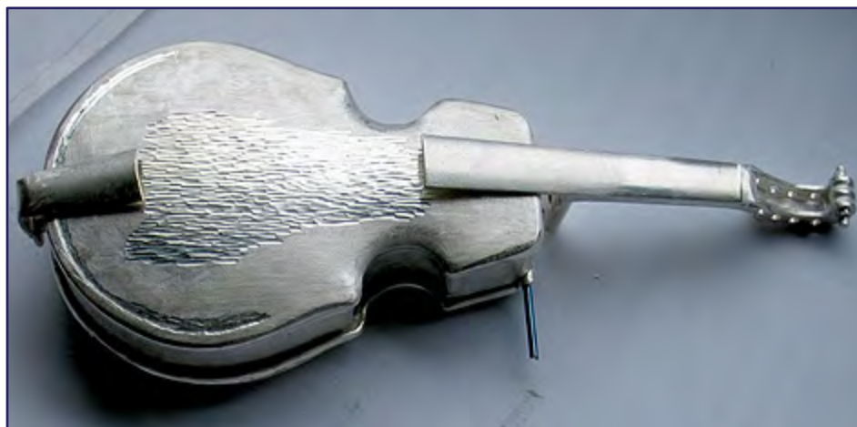
5. Engraving in progress on body face within the engraved recess around the edge.
