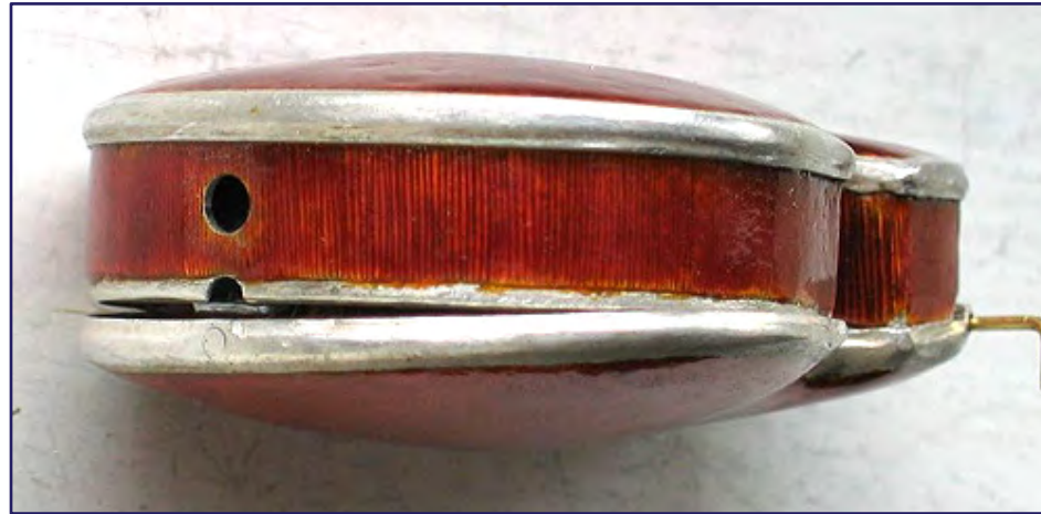
9. Distortion of the back, prior to correction.
