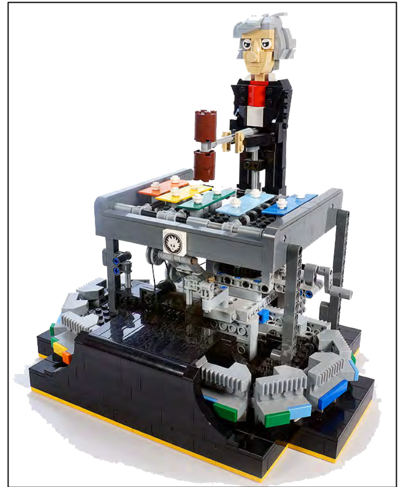
3. LEGO glockenspiel automaton ( Ludwig version). Apart from the xylophone pieces, this amazing model is 100% LEGO. When the crank is turned, Mr. van Beethoven bangs out the main "Ode to Joy" theme from his Symphony No. 9. His movement is timed and "programmed" by means of an ingenious, colorful rotating chain at the bottom.
