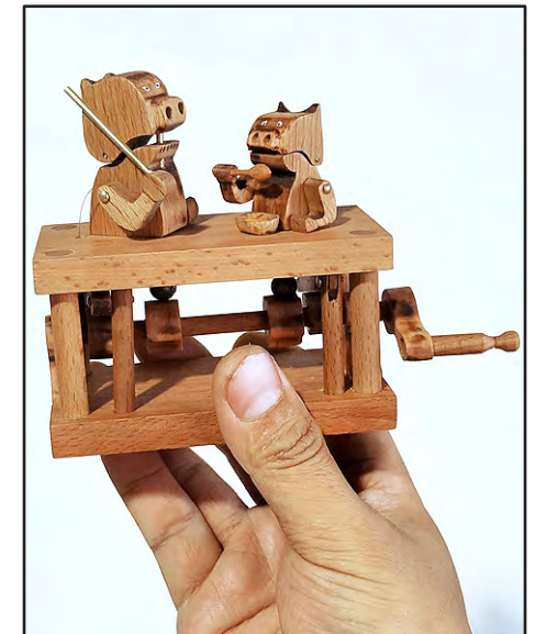
3. The cams are stuck on this one.
