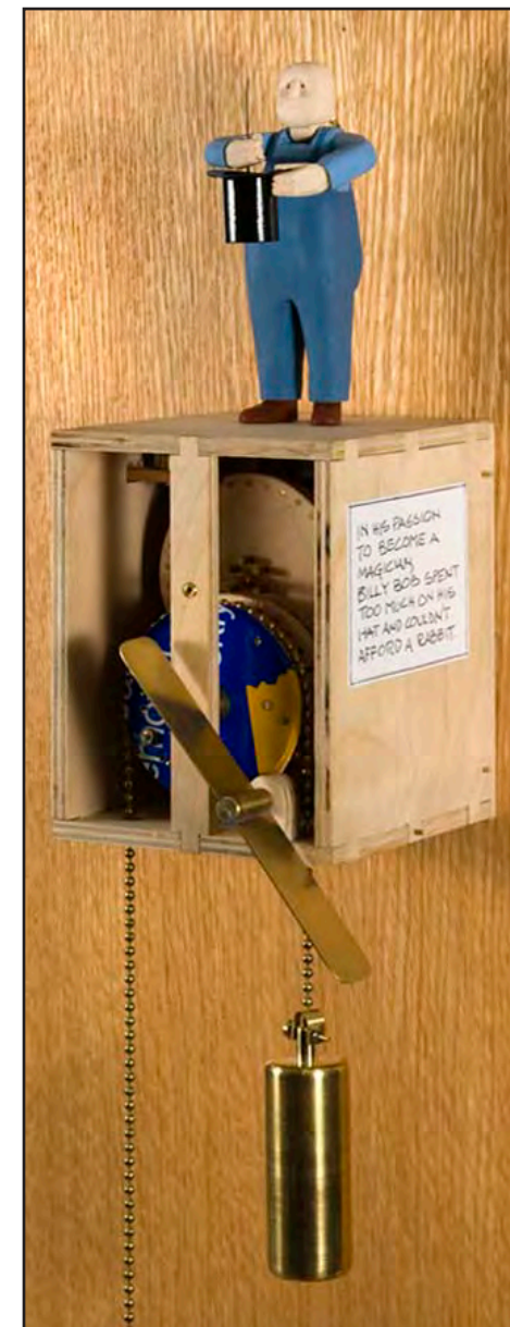
This automaton, which was also produced in hand-crank form, is mounted to the end of a bookcase. The piece is powered by the weight hanging from it on a chain.
