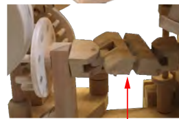
See the joint opening up as the front axle connection moves away from the driveshaft.
