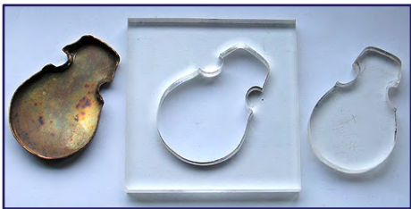
2. Acrylic-plastic profile and trial pressing in gilding metal.
