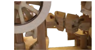
Notice how the different parts of the joint can twist and turn at different angles to each other.
