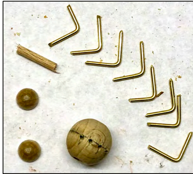
1. The parts to make a baby spider. The wooden ball that forms the body has been predrilled to accept the legs.
