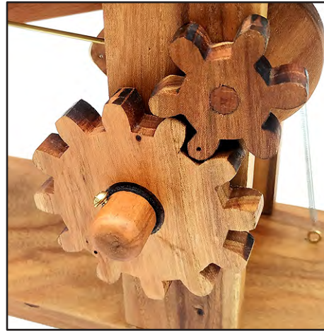
4. Wooden gears can bind and lock if they become deformed.
