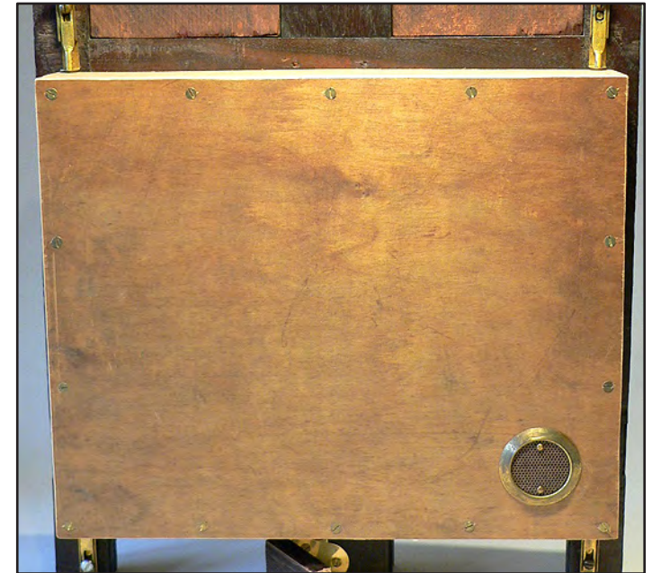
11. Rear view, with the cover on. Speaker grille is at lower right.
