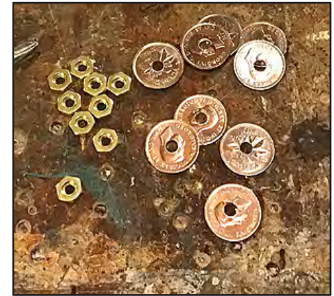
3. Canadian pennies soldered to brass nuts form the pipe ends.
