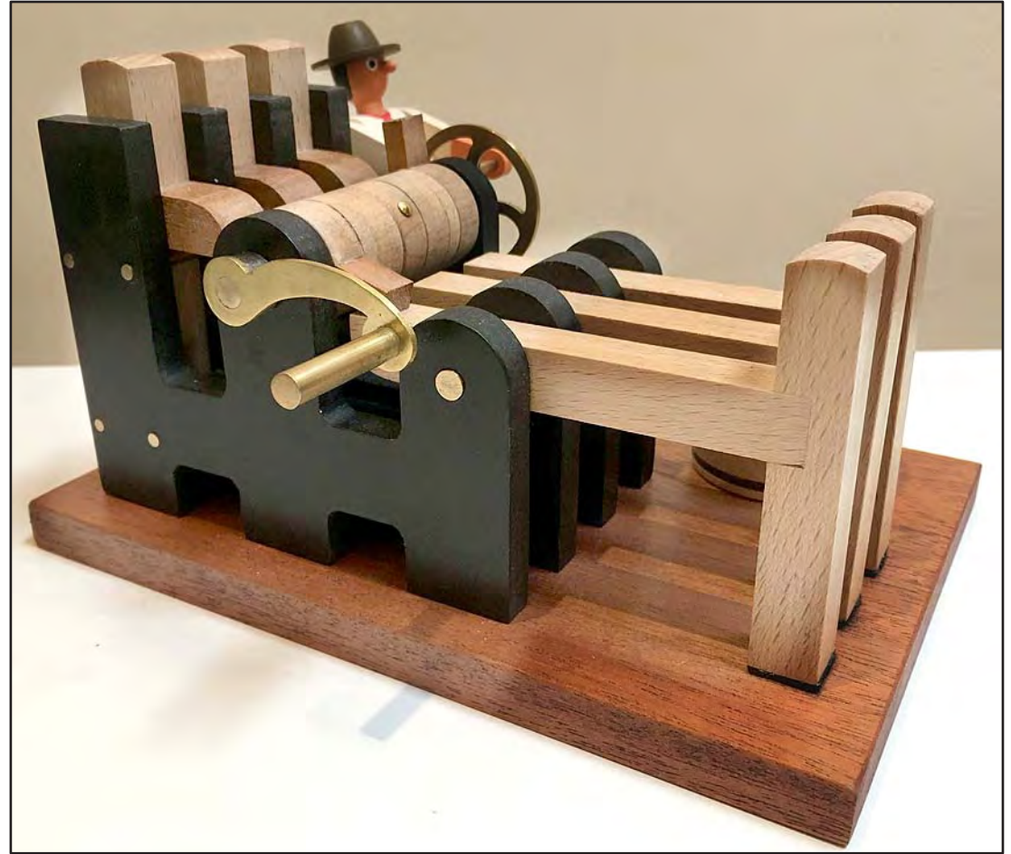
RIGHT: 5. The finished fulling mill. This is the side from which the observer cranks the machine.
