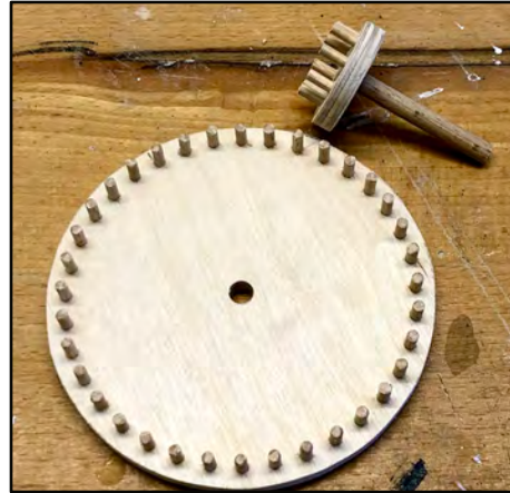
4. The two pinwheel gears, one eight tooth and the other thirty-six.
