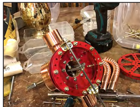
8. The drive mechanism for the siphons.
