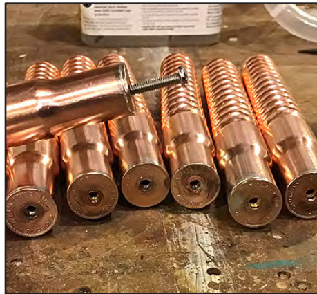
4. Finished threaded pipe ends with the pennies in place.
