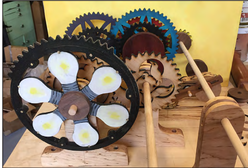
1. Gears and axles have been placed on the floor of the automaton to help determine their proper location.
