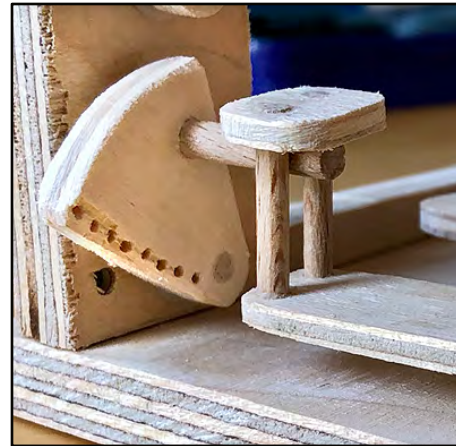
9. A bell crank, driven by the cam-follower, changes the direction of motion.
