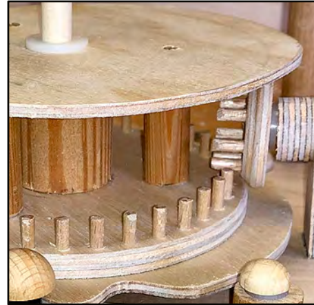
5. Pinwheel gears engaging. The arm cam is above, the mouth cam below.
