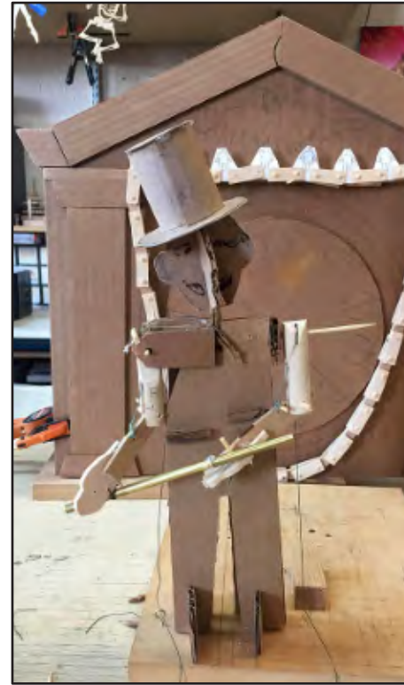
5. A preliminary cardboard prototype was made to work out the mechanism for raising the flute to the magician’s mouth.
