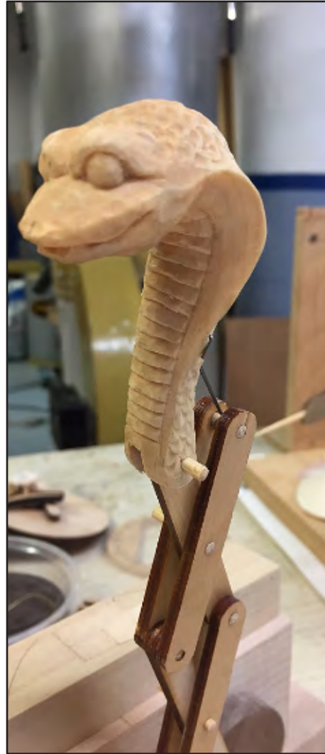
7. The snake rises from its basket via the action of the scissor arm, seen here. The author hand carved the snake's head.
