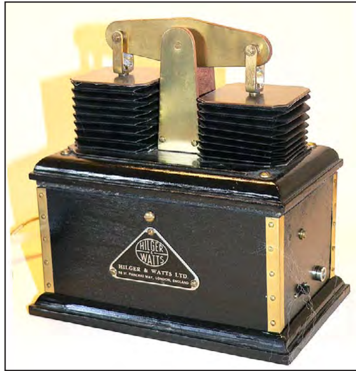
3. The air-pump unit. The bellows were made of a repurposed photographic lens extension.
