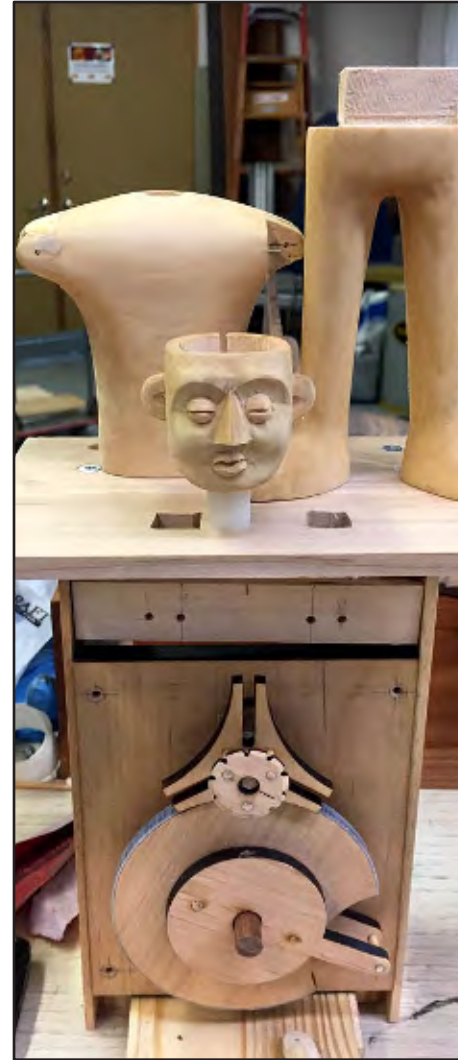
8. The three-position Geneva mechanism, under construction. Above are hand-carved head and body parts.
