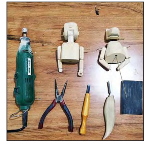
7. Figures were carved and shaped from wood, with knives, a rotary tool, and sandpaper.
