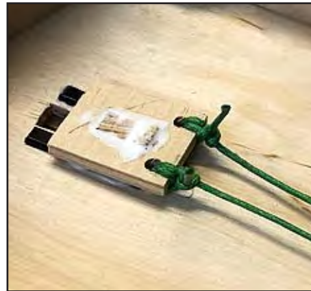
2. The underside of the sliding nose. Strings attach to the spring-loaded mechanisms for the eyes and ears. When the nose is slid forward, the eyes and ears are activated.
