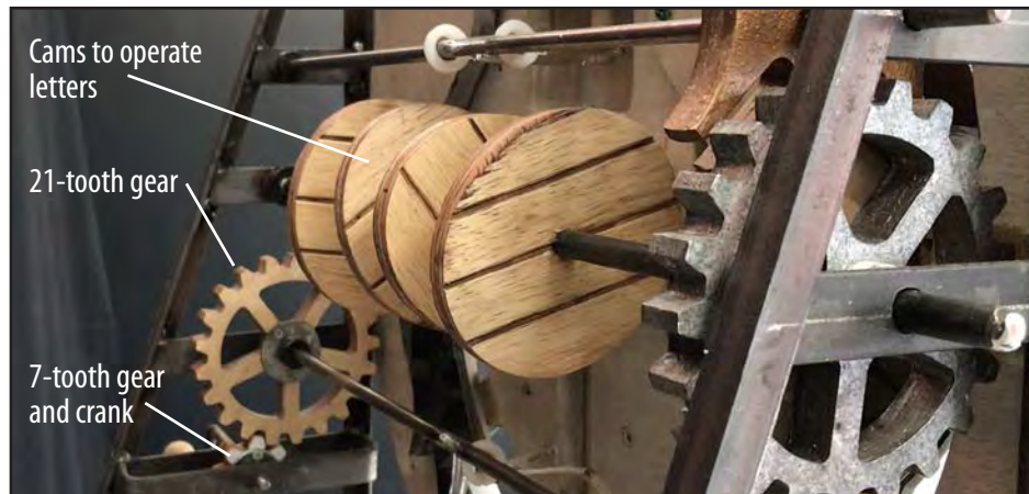
8. The mechanism that powers the action. The four different shafts, starting from the bottom, can be seen in this photo. Gears and cams are made of plywood.
