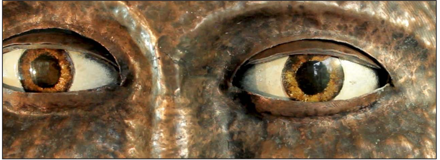
7. The automaton's eyes, made primarily of plastic and resin, slowly open and close as the cycle progresses.
