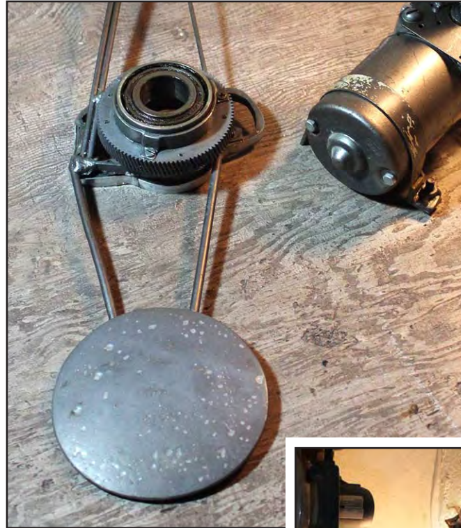
10. The lead counterweight on the arm assembly, with the central car-wheel bearings.
