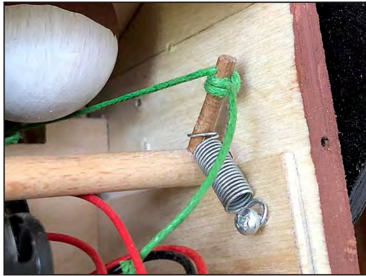
6. Behind the eyes is the spring-loaded lever that activates the ears. The second string from the nose is in place.
