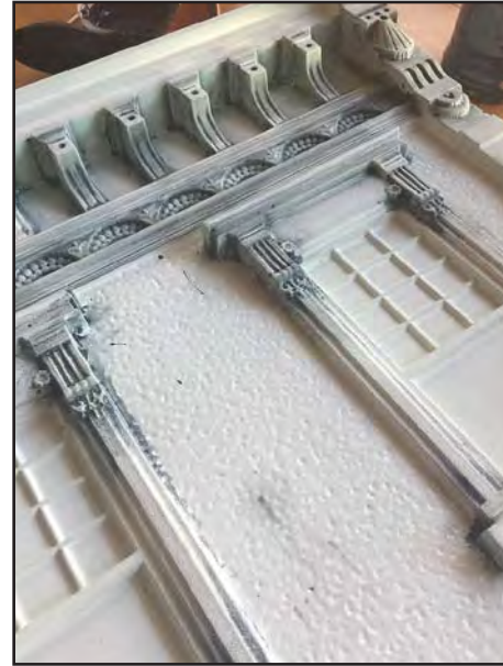
LEFT: 4. A wall being finished. After the carving was done with the computer-controlled router, the walls were painted and weathered.
