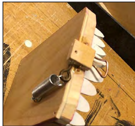
8. The wire latch that holds the jaws closed is released when the nose is pushed forward. The spring keeps the latch closed until the nose is moved.
