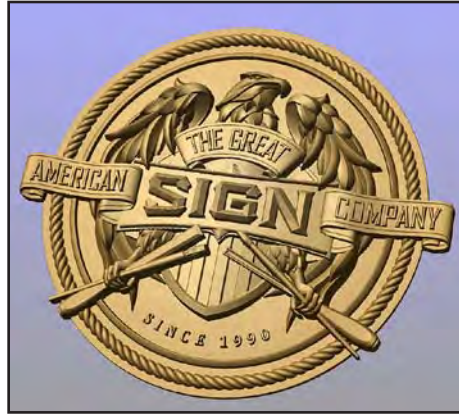
LEFT and ABOVE: 2 and 3. Computer drawings of a wall of the building and the company's logo. These designs would be rendered in high-density urethane foam by a CNC router, then backed with plywood.
