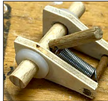
3. The eye mechanism. Eyeballs will be fixed to the dowel ends. Plastic washers reduce friction. The activating string will be attached to the lever.
