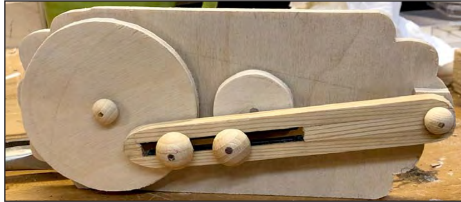
2. The basic mechanism. The small central wheel is turned by the crank on the outside of the partition, causing the big wheel at the left to rock back and forth. Note the black plastic strips in the slot to reduce the friction. These are cut-down tie wraps.
