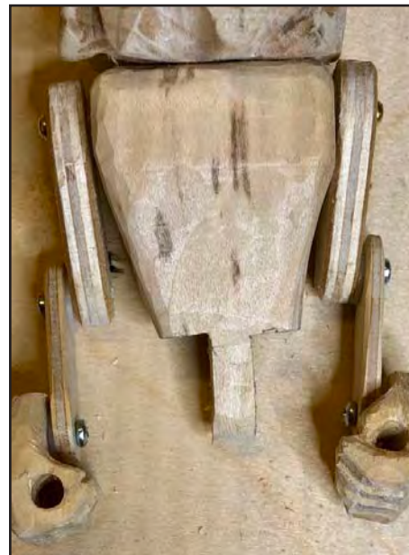
9. The arms, hinged with screws and plastic washers, and the hands that will hold the swing's axle ends.
