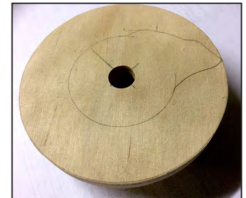
6. A marked cam, ready for cutting.
