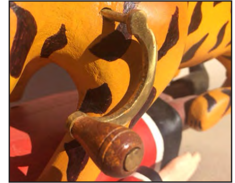
2. The author crafted the crank from brass and turned the wooden handle on his lathe.
