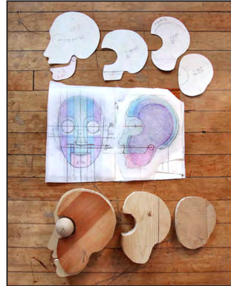
2. The head armature is made of 3/4"-thick pine layers, cut and glued together, then carved to the head shape. The jaw part and wooden balls for eyes are separate, and they will be jointed using metal pivot rods.
