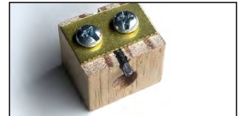
4. The pencil block, which temporarily replaces the follower bearing for marking.
