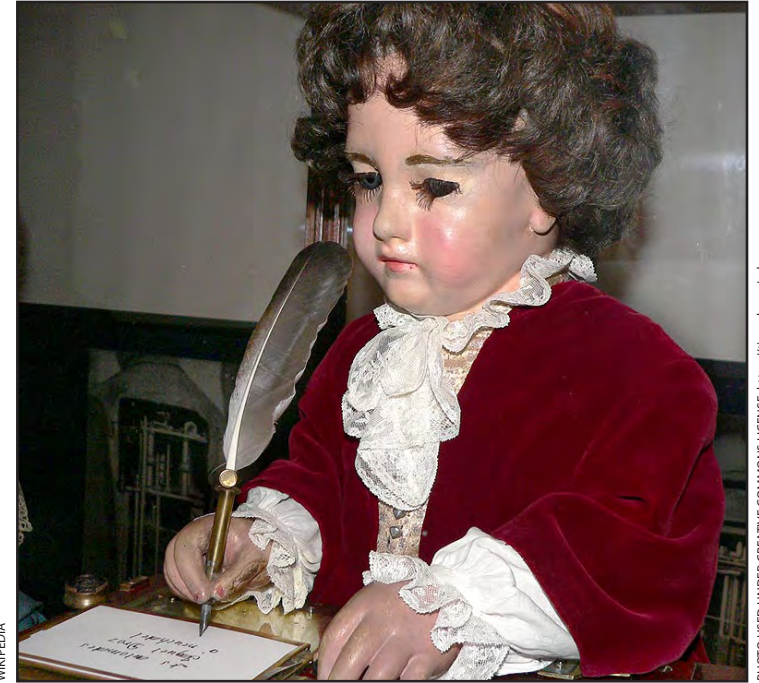
2. Pierre Jaquet-Droz’s automaton, The Writer , is able to pen any text up to 40 characters.
