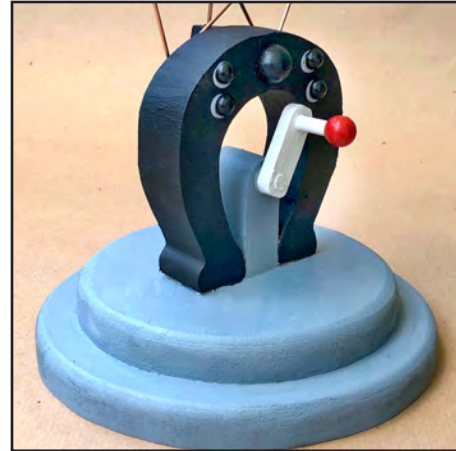
4. The finished base, viewed from the crank side. The horseshoe shape forms a frame for the mechanism.
