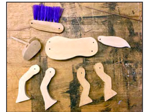
2. The cut-out pieces of the unicorn, ready for painting and assembly.
