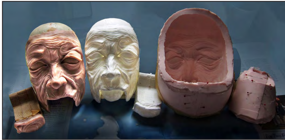
7. A silicone-rubber mold was made of the old face and the separate jaw. These were then cast in two-part resin. Left: Super Sculpey model. Middle: resin casting. Right: face and jaw molds.
