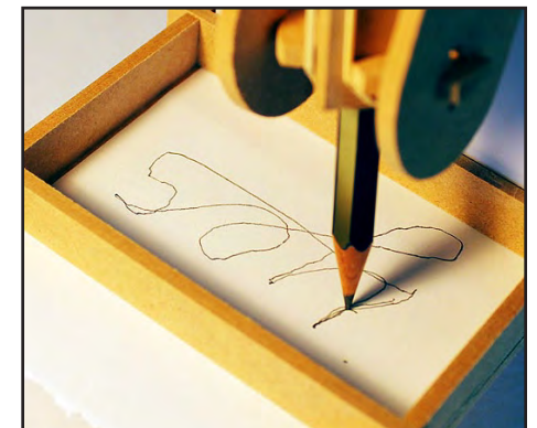
6. “Yes,” as written by Scriblo on its writing pad. The paper is on a roll. Once written, the word can be pulled out and torn off the roll.
