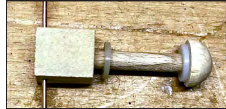
ABOVE: 9. A small hemisphere on the dowel prevents the rod (not shown) from coming off. Plastic washers reduce friction.
