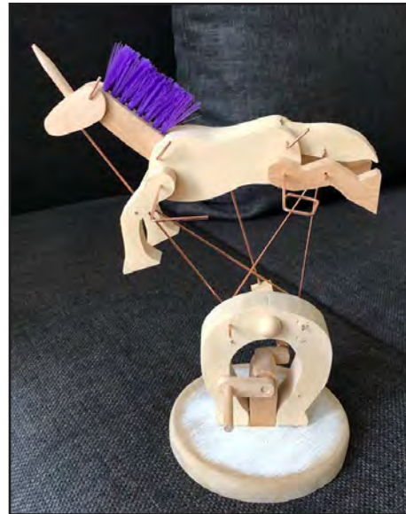
11. The unicorn, assembled but unpainted, ready for testing. Note the bent-wire "handles" left on the ends of the pivot-pin rods. These will be trimmed off when everything is working properly.
