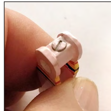
5. An example of a shortened screw. A new slot has been saw-cut into the threaded body of the screw.
