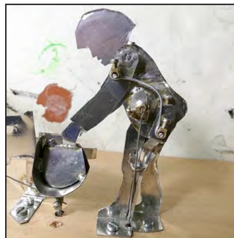
4. Extensive use of halved terminal blocks has been made in this automaton, shown from the back. Video: https://youtu.be/rN1_bmsgl7M
