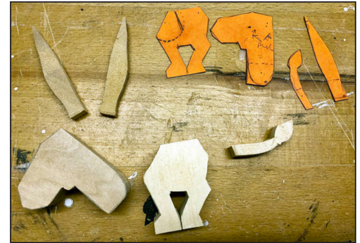
3. Parts are cut from wood on a scrollsaw.
