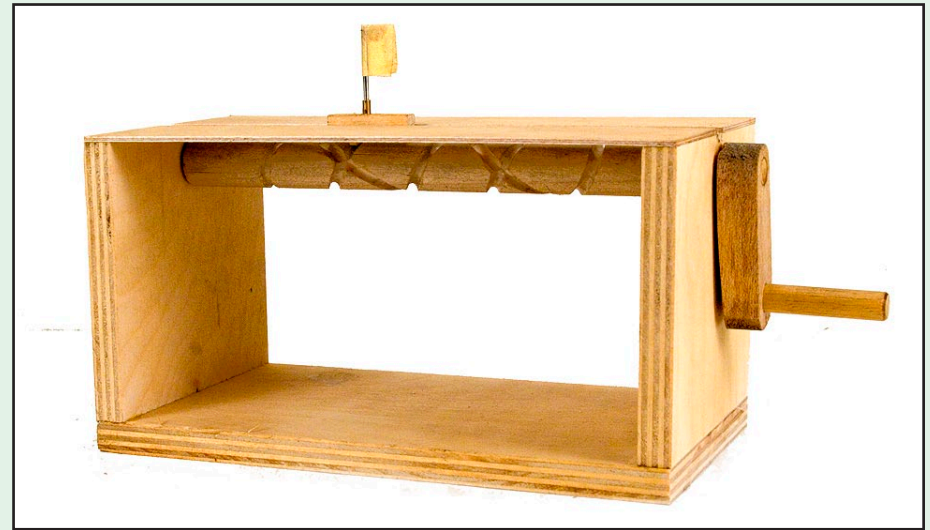
The finished mechanism. The little flag on top indicates where the follower is pointing.
