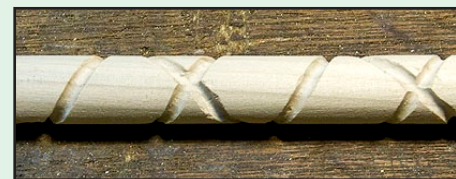
10. After being filed, the semi-finished groove.
