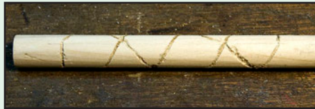
7. The rough dowel after sanding off the burrs.
