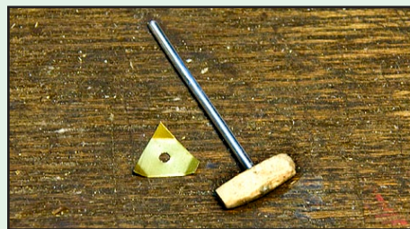
14. The new wooden follower with the brass spring.
