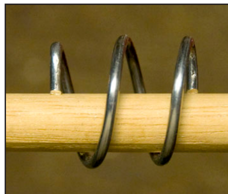
11. The wooden shaft is slid into the helix below the cut ends.
