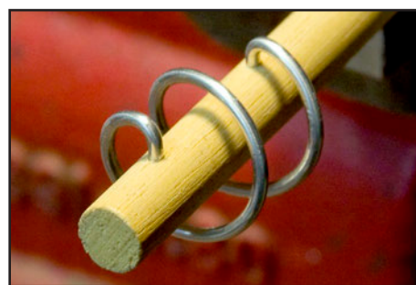
14. The helix, mounted on its shaft prior to centering.
