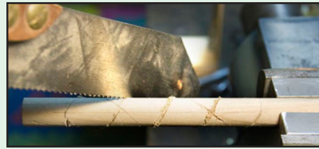
6. Initial cutting of the groove with a saw.
