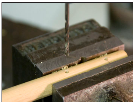
13. Drilling the holes.
