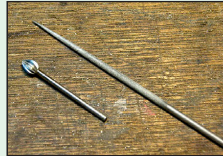
9. The Dremel bit and the file used for additional grooving.
