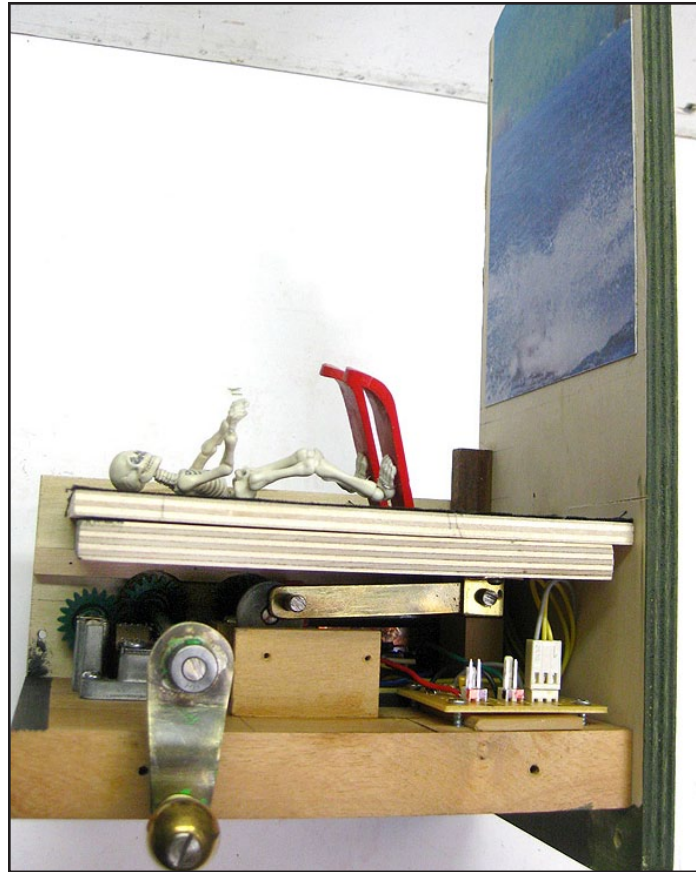
7. The bottom plate oscillates while the top plate, with the skeleton, slides with it. When the top plate hits the stops, its motion pauses.
