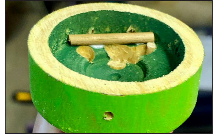
12. A circular wooden base the author had on hand was used for the donkey to stand on. The round dowel inside eases the path of the cords.
