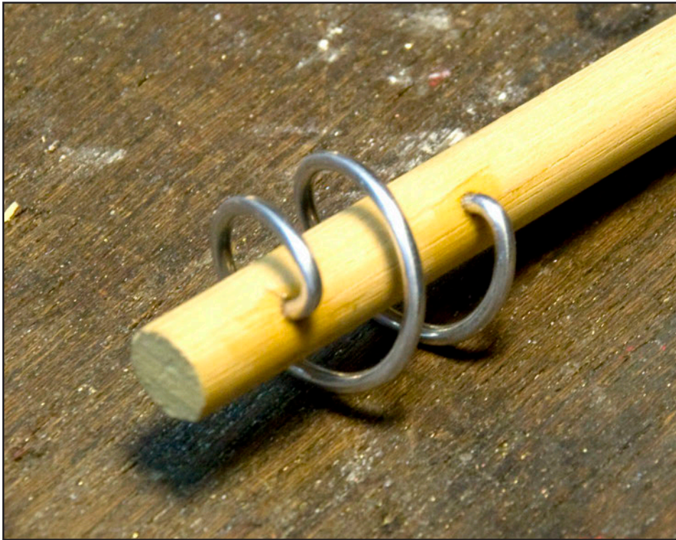
16. The finished assembly, with the helix centered on the shaft and glued in place.
