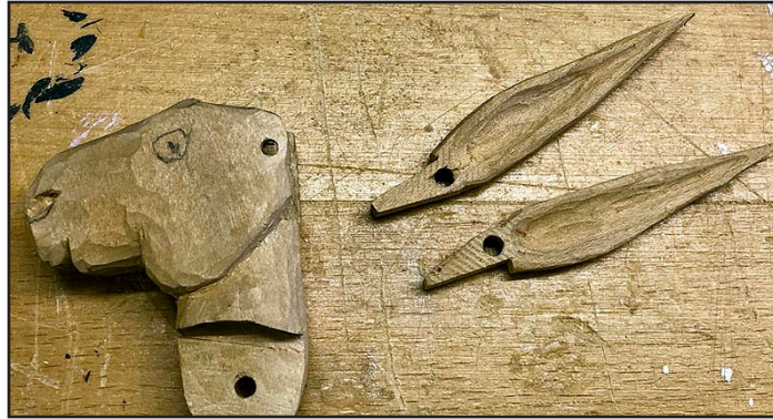
6. The ears and head, carved to their final shapes. Pull-cord holes have yet to be drilled in the ears.
