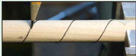
3. Marking the dowel along the thread.
