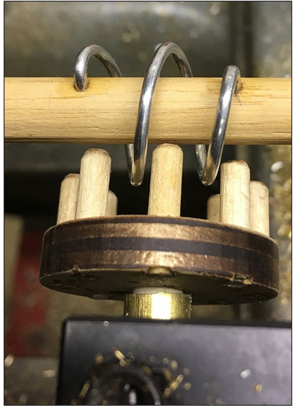
17. The worm and pinwheel being tested in the lathe.
