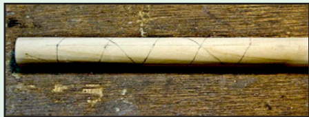
5. Both helices are marked on the dowel.
