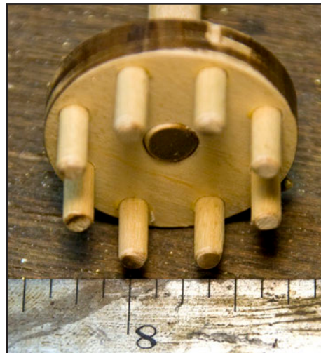
1. The pitch (distance between the teeth) of this pinwheel is \frac{3}{8} " (9mm).
