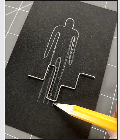
23. Drawing the figure on paper. Leg spacing is made to match the crankshaft.
