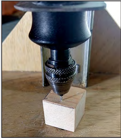
27. The block is drilled for a rod that will be inserted into the hole to support the figure while it's walking.
