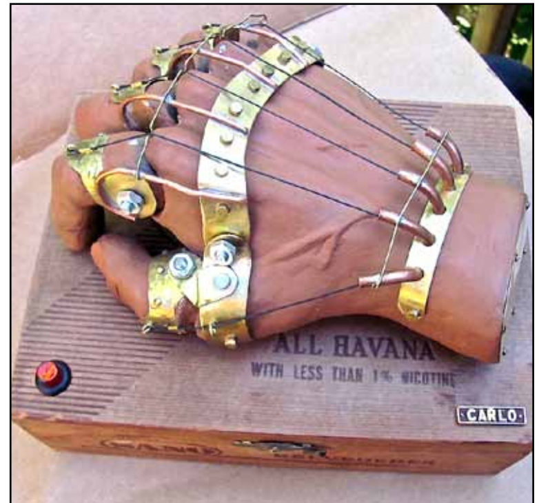
4. Though all fingers appear mechanical, only the index finger actually moves.
