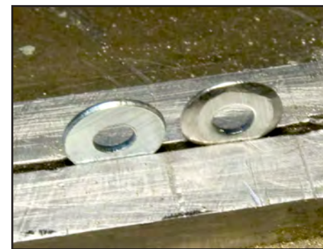
3. The right-hand washer has been filed, its edge smoothed and thinned.
