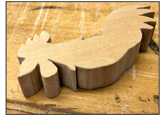
2. The body of the chicken has been rough cut on the scroll-saw.
