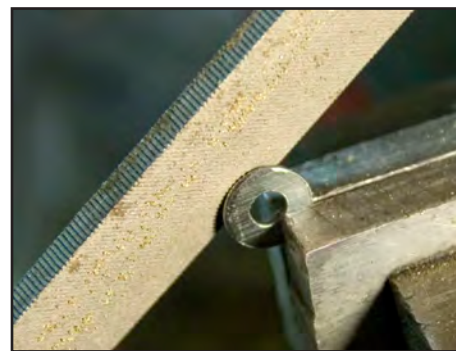
2. The outer edge of the washer is filed on both sides.
