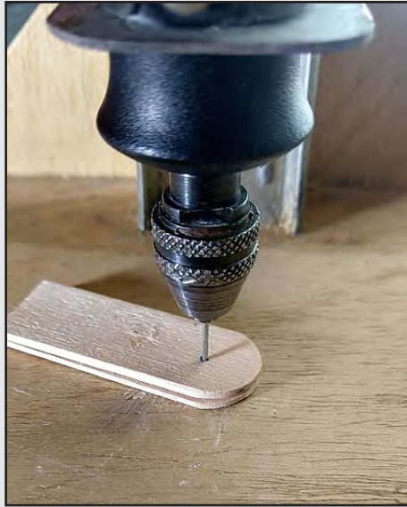
21. Crank holes are drilled in both pieces together, for accuracy.
