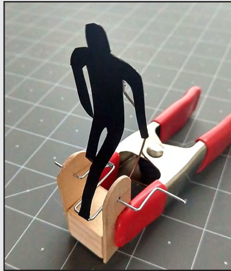
28. A clamp temporarily holds the piece together for a dry run. Note the wire in back holding the figure up.
