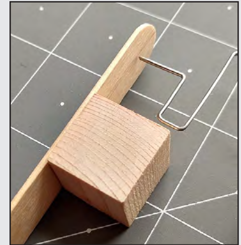
17. The bent wire is used as a guide to determine the length of the side piece.
