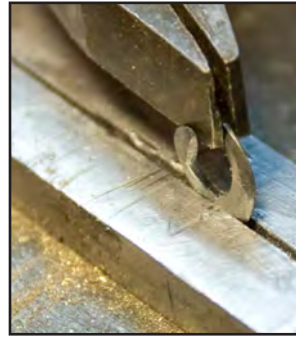
6. Legs are bent parallel to each other.
