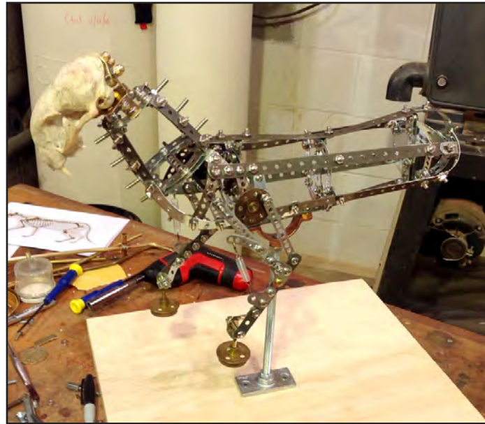
2. The forelegs, with mechanical linkages in place.
