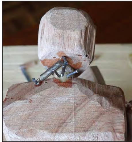
9. Fishing line (just visible) is attached to the figure's head and lower body. When he bends, the line causes the head to turn. The spring returns it to its former position.
