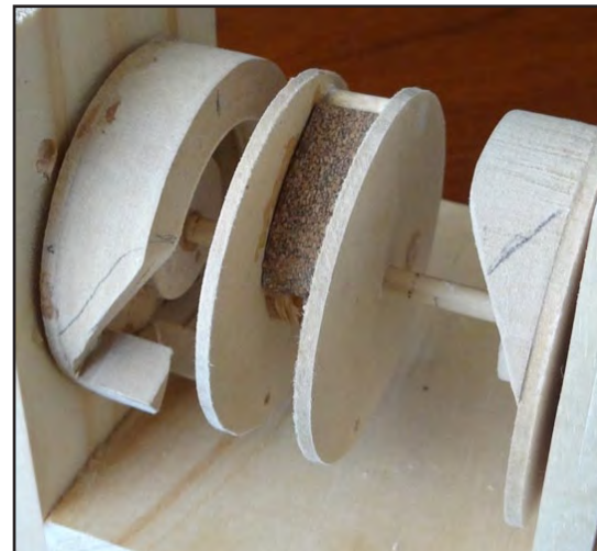
LEFT: 7. A wooden, waist-level hinge, made of dowel segments and mounted diagonally through the cross section of the woodworker's body, allows the figure to lean forward in a more natural manner.
