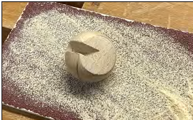
6. Head sanding was done on coarse paper laid flat.
