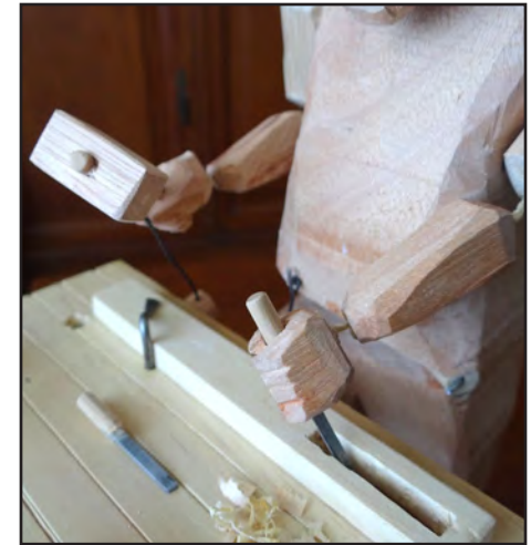
11. The mallet and chisel are held in the hands by friction. The hole in the chisel hand was later enlarged so that the chisel would move freely, making the motion more natural.
