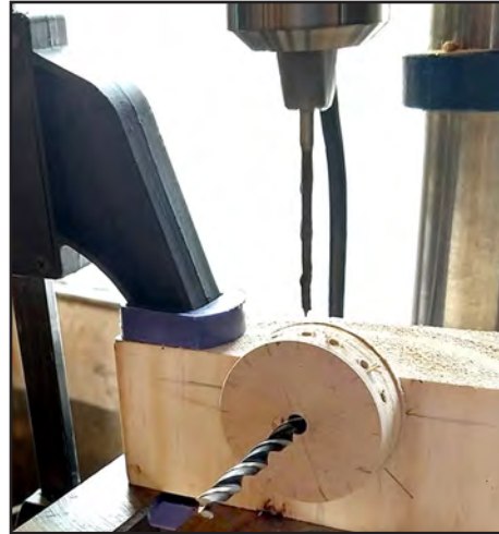
6. An MDF gear blank being drilled for the pins, in the author's drill press.
