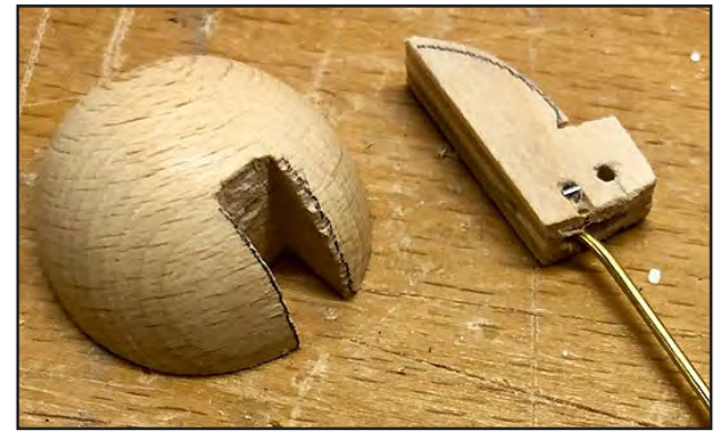
8. The plywood hinge piece with the pushrod in place.
