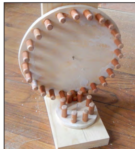
Pre-checking pinwheel gears on a separate scaffold. The author uses a gear-template generator to help mark the pin placement.
