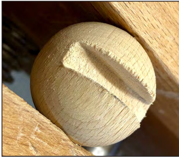
4. A slot for the plywood hinge has been made in the head.
