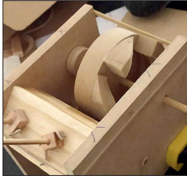
ABOVE: 3. This wheel controls the mallet striking the chisel.
