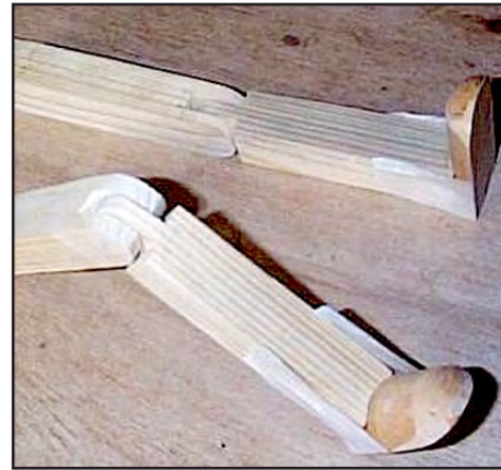
2. Note the simple but effective knee-joint hinges on the legs.
