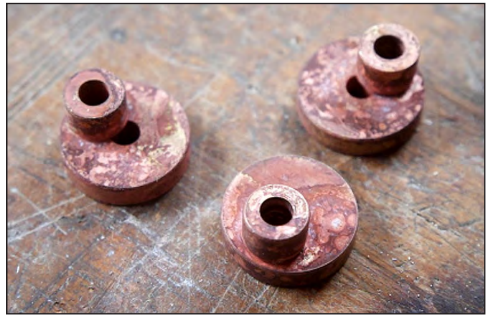
4. Cams were each made from two pieces of brass, silver soldered together.
