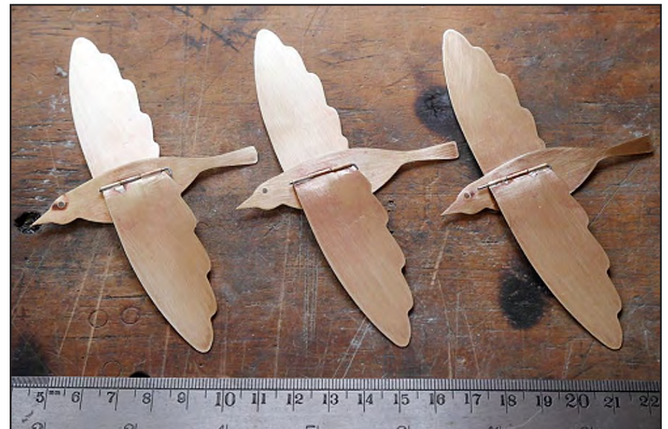
2. Wings are attached to the bodies by hinges constructed of brass tubing.
