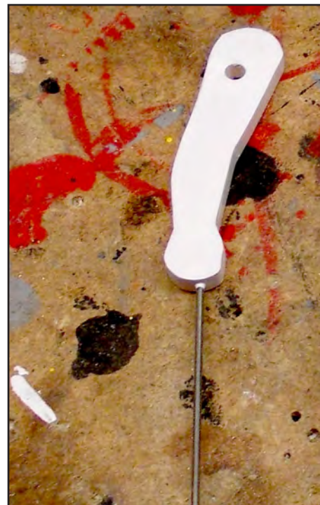
4. Hole drilled into the edge of the Perspex and the foil inserted.
