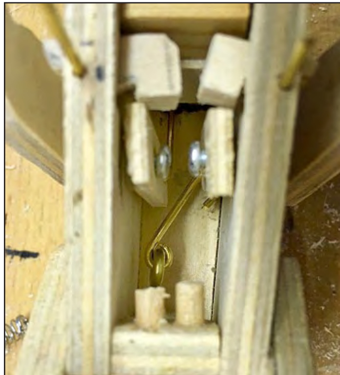
5. A front leg with its hinge, which will be glued into the marks.
