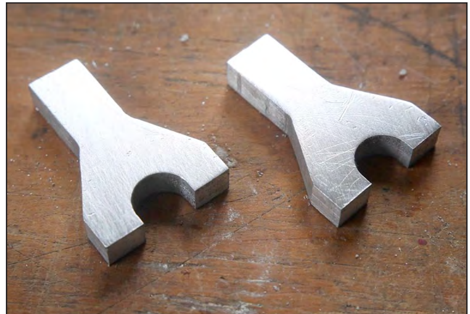
3. These two pieces, milled from aluminum, form the base of the mechanism.
