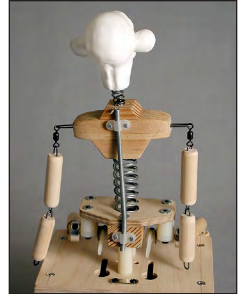
3. A balancing-spring spine solved the drooping problem.
