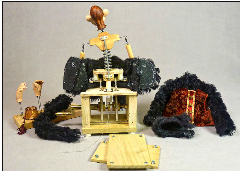
11. Jayfred , ready for final assembly. He's made of wood, springs, brass, resin, and epoxy clay. He has glass eyes and hand-painted hands, head, and feet. His hide is black mohair fabric. Jayfred's 14"-long tail has a braided-wire armature inside, bendable to any position.
