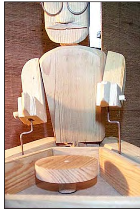
8. Controlled by cams from below, the potter's arms raise and lower simultaneously to simulate the throwing of a pot.
