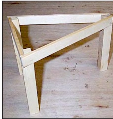
5. Three-legged base for the potter's wheel.
