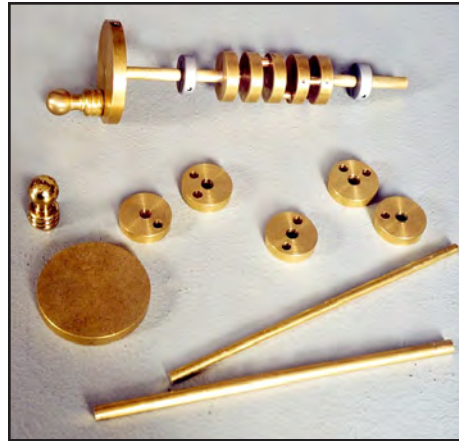
5. An assembled crankshaft (top) and all the necessary parts for another. Crankshaft parts are made of brass and must be made with great precision.
