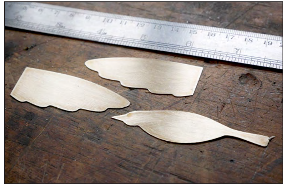
1. The bird's body and wings were cut from brass sheet on the author's homemade CNC router.
