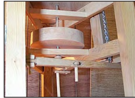
6. The wheel's kick mechanism. The main shaft comes up through the floor, powering the wheel itself. The large wooden flywheel can be seen here. A crank on the shaft actuates the foot-power mechanism.
