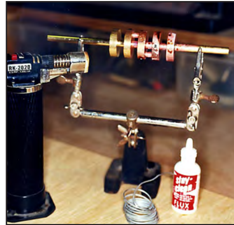
6. The crankshaft is held in a "third hand" for silver soldering. The central axle will be cut out to form the separate cranks.
