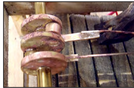
15. Motion is from a crank axle geared to the treadmill and wheels, and wired to the legs.
