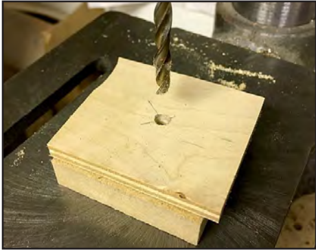
23. A hole the size of the center plug is drilled into the wood.
