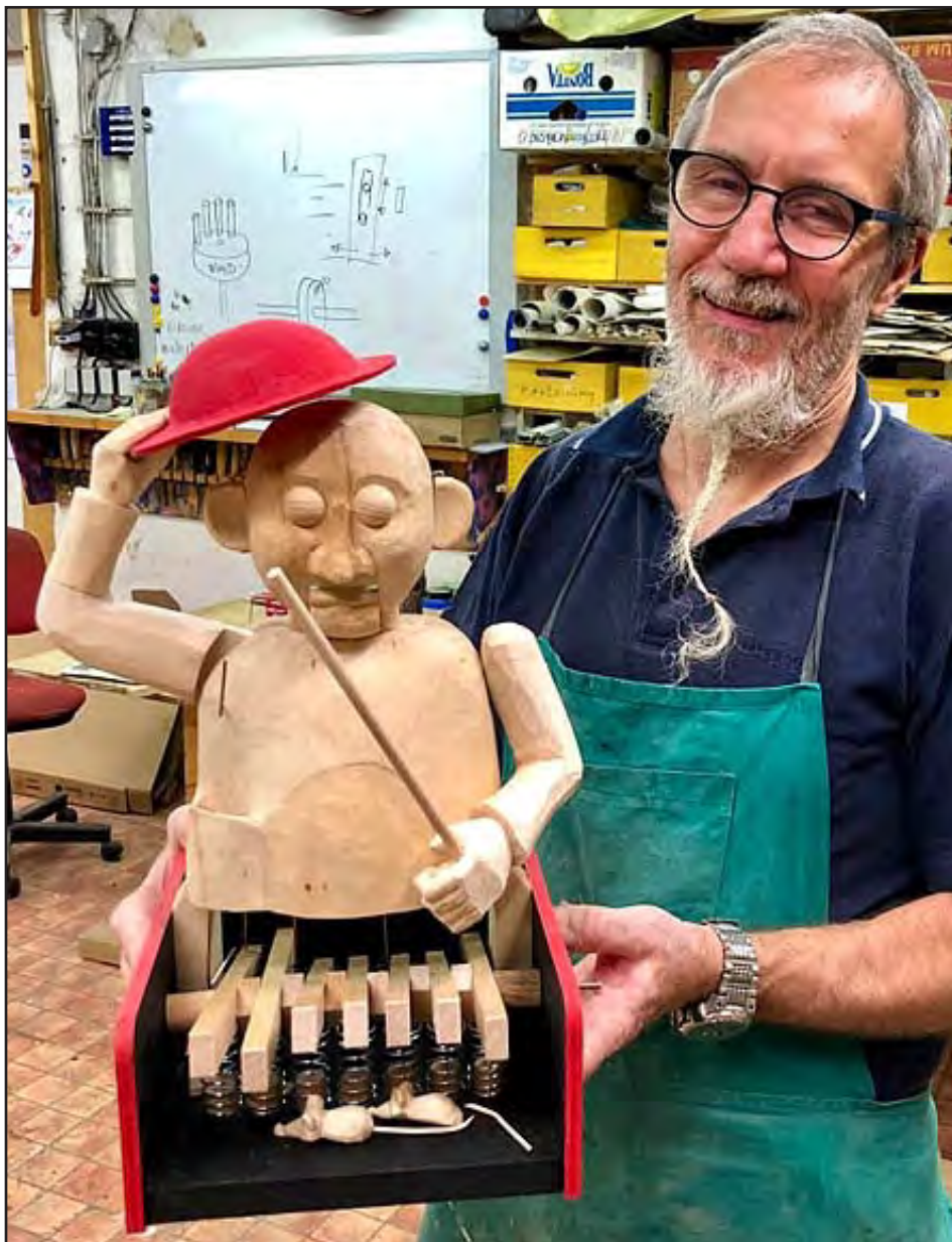
The head has been screwed to the body, which has been screwed to the base, and the mechanisms are starting to be fitted. Here, Zdar holds the author's automaton in its nearly complete state at the end of the course. The piece was finished by the author after returning home.
