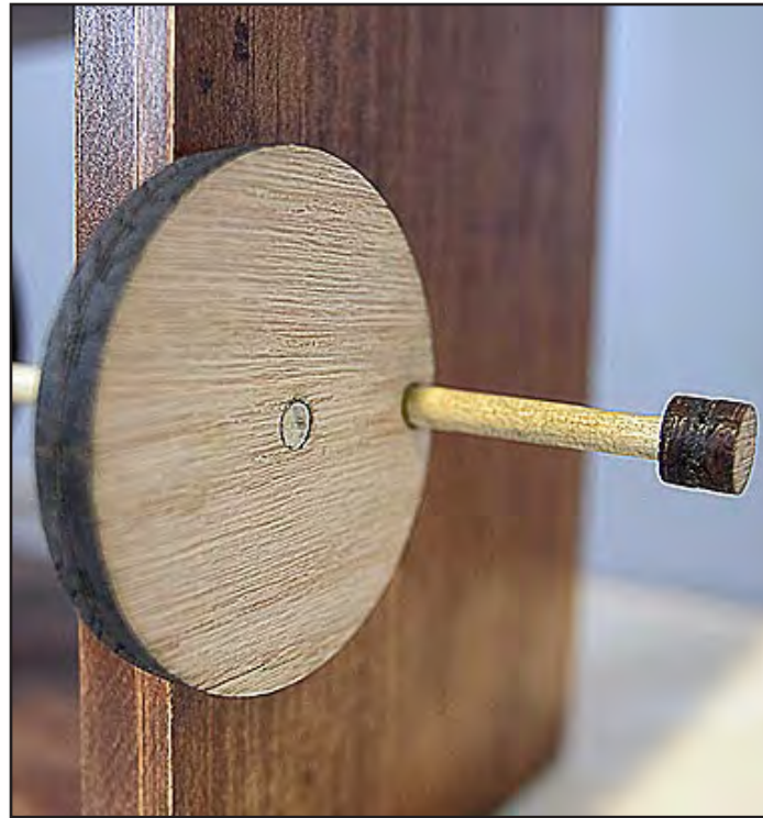
10. Laser-cut crank handle. The dark, burned edges are characteristic of the process.
