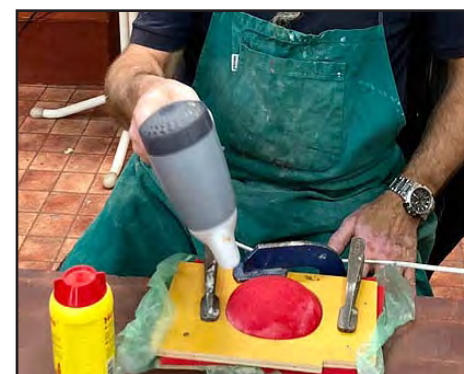
Zdar making a hat from two layers of felt soaked in glue.
