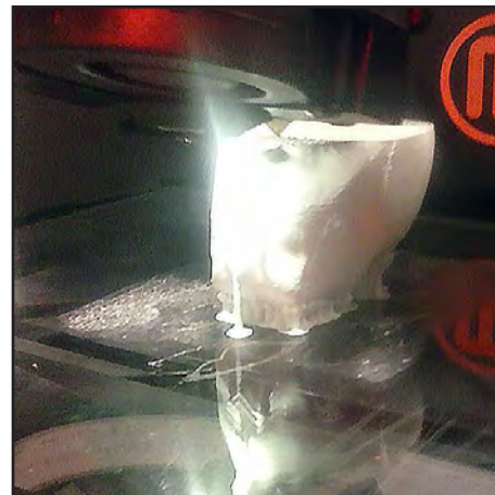
4. A head in the process of being 3D printed in plastic.
