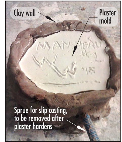
7. A two-part plaster mold was made to cast a smooth head.
