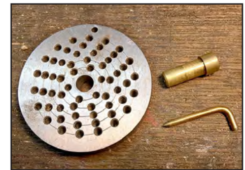
22. The three parts of the tool: the plate, the center plug, and the pointed pin.
