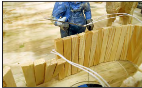
8. The slats were threaded onto loops of sail-maker's thread.
