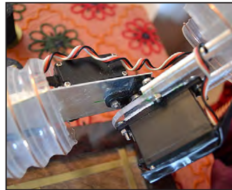
8. Shoulder and elbow servos provide motion. The second elbow servo works the hand.
