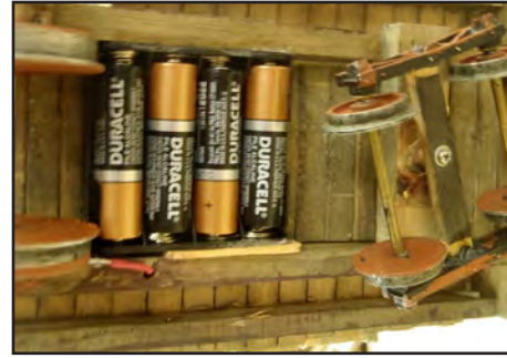
17. Power to the reworked R/C servo is supplied by four AA-cell batteries under the floor.
