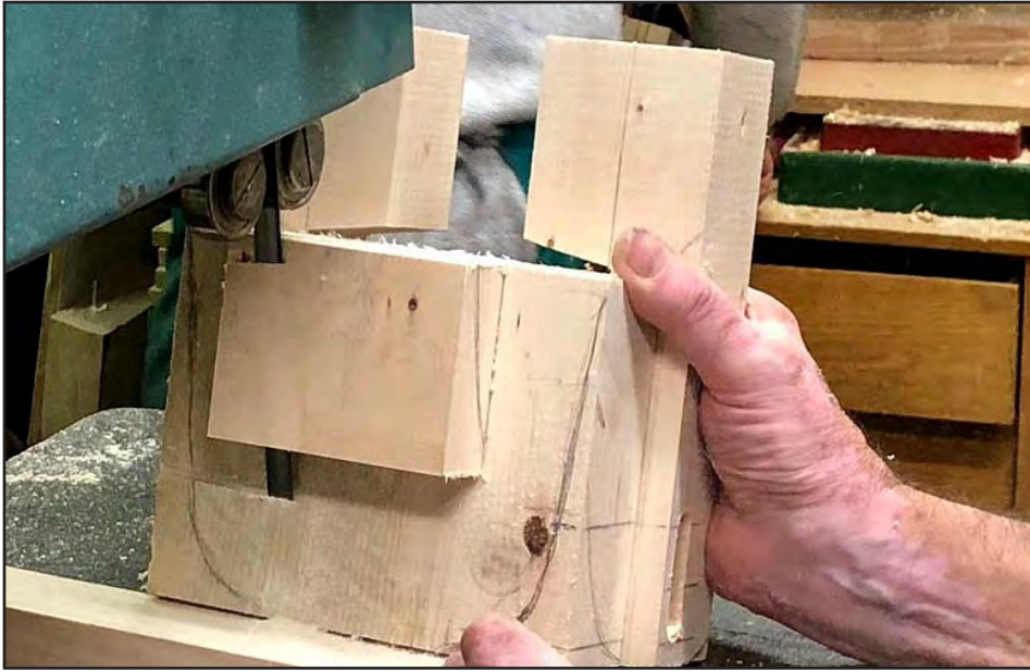
The glued-together, blocked-up body, which dried overnight, being trimmed roughly to shape.
