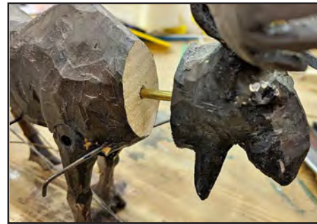
20. In order to make Moose’s head waggle, it had to be amputated and reattached. A brass rod nesting in a tube allows a rocking motion.
