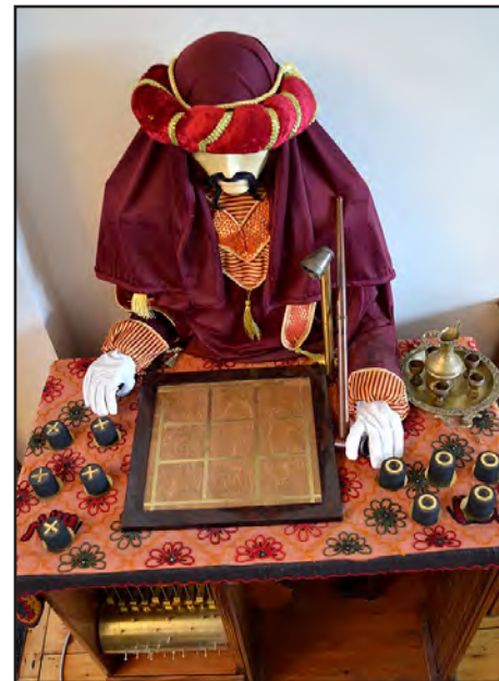
2. The author's Turk plays noughts and crosses (tic-tac-toe). Playing pieces are bits of curtain rod with brass X's or O's glued on top. The board is a picture frame with a plywood insert, trimmed in brass.
