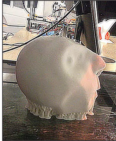
5. The finished head still on the printer bed. The support pieces underneath will be trimmed away.
