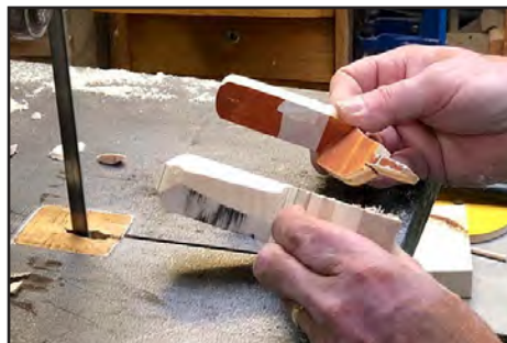
Cutting the left arm on the bandsaw from the maquette.
