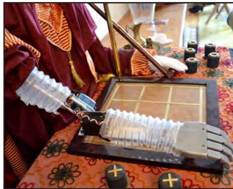
7. Flexible wire-reinforced plastic tubing gives the Turk's arm shape and form.
