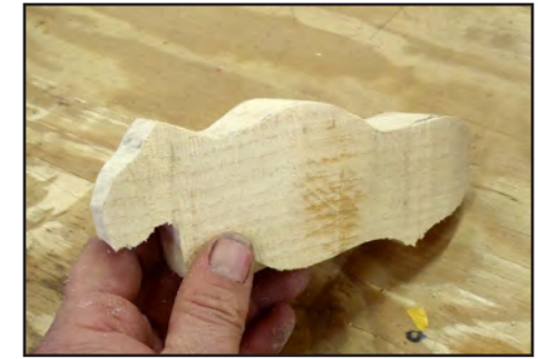
3. Moose himself was freed from a piece of pine, using the bandsaw, then carved to shape with chisels and a sharp knife.
